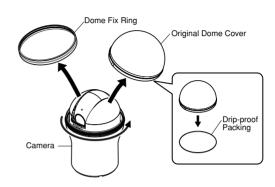
Replace the dome fix ring removed in Step 2, and turn it to the right until it is tight.
