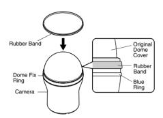
Place the drip-proof packing removed in Step 2 onto the replacement Dome cover WV-CS3S, and put them on the camera.
