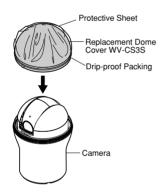
After turning the dome fix ring to the left, remove the original Dome cover from the camera, and then remove the drip-proof packing.
